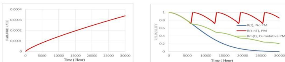
Figure 5. Failure rate Servo Fuel Heater (a), PM on Servo Fuel Heater (b)
