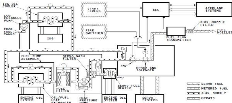
Figure 2. Diagram Blok of Engine Fuel and Control system
