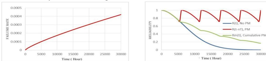
Figure 4. Failure rate on IDG Oil Cooler (a), PM on IDG Oil Cooler (b) Servo Fuel Heater, The data failure or TTF dispersion pattern of the Servo
