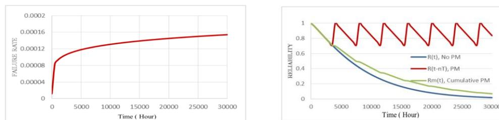
Figure 3. Failure Rate on Fuel Pump (a) and Implementation PM (b)
