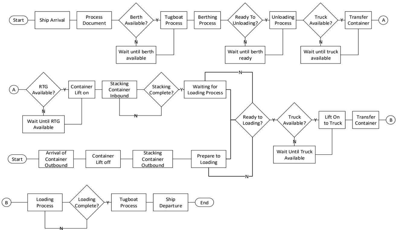
**Fig. 6.** Simulation Flowchart
