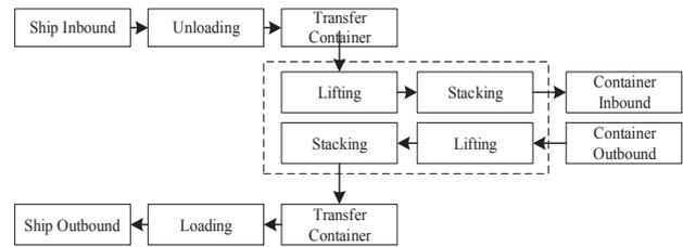
Fig. 3. Operation Process at Container Terminals
