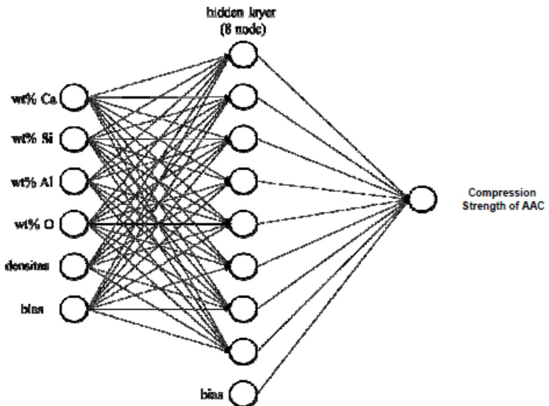
Figure-3. Artificial neural network architecture
