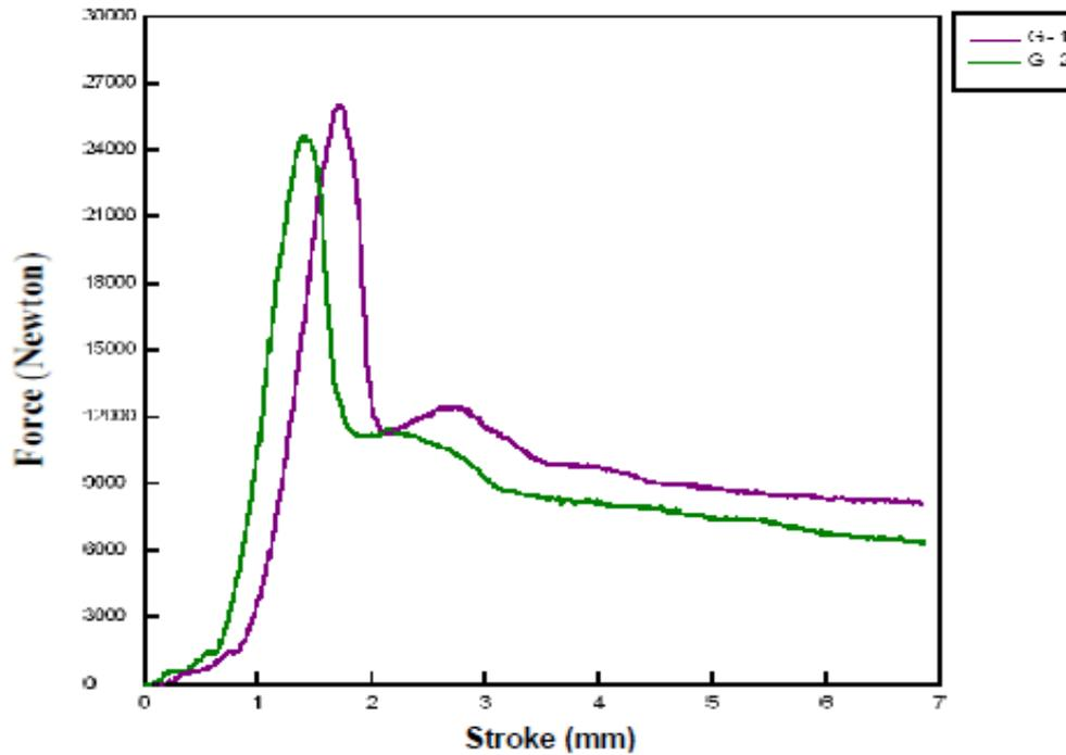
Figure-2 : Sample AAC result of mechanical test
