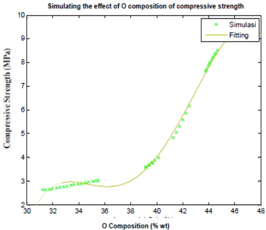
Figure 7. Simulation results of the effect of wt% O on compressive strength
