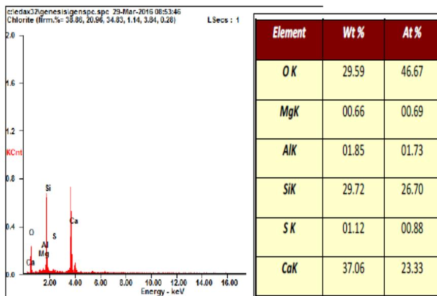
Figure-1 : Sample AAC result of composition test
