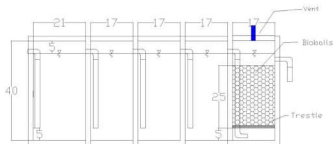
Figure 1. Reactor A with anaerobic-anaerobic processes
