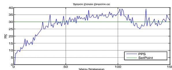
Fig 11. System response to a set point of 30 pps.
