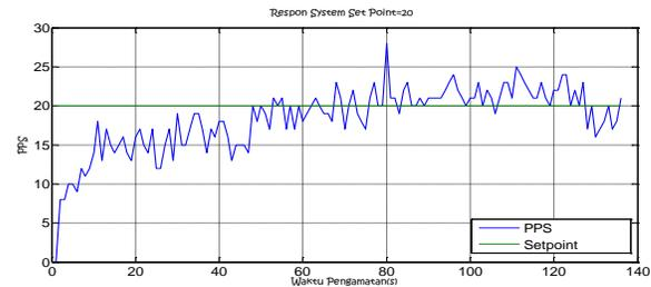
Fig 10. System response with a set point of 20 pps
