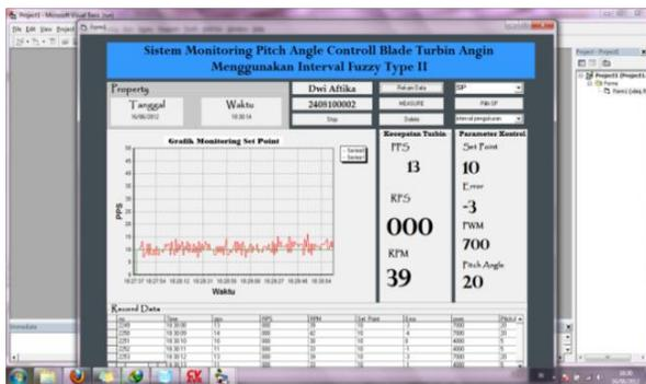
Fig 8. Interface monitoring system controls the pitch angle of the wind turbine
