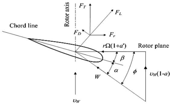
Fig 1. Vector force on the turbine blade [1]
