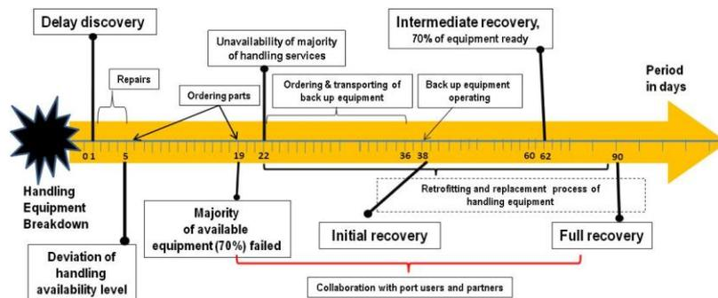
Figure 2: The cases of port congestion due to handling equipment breakdown
