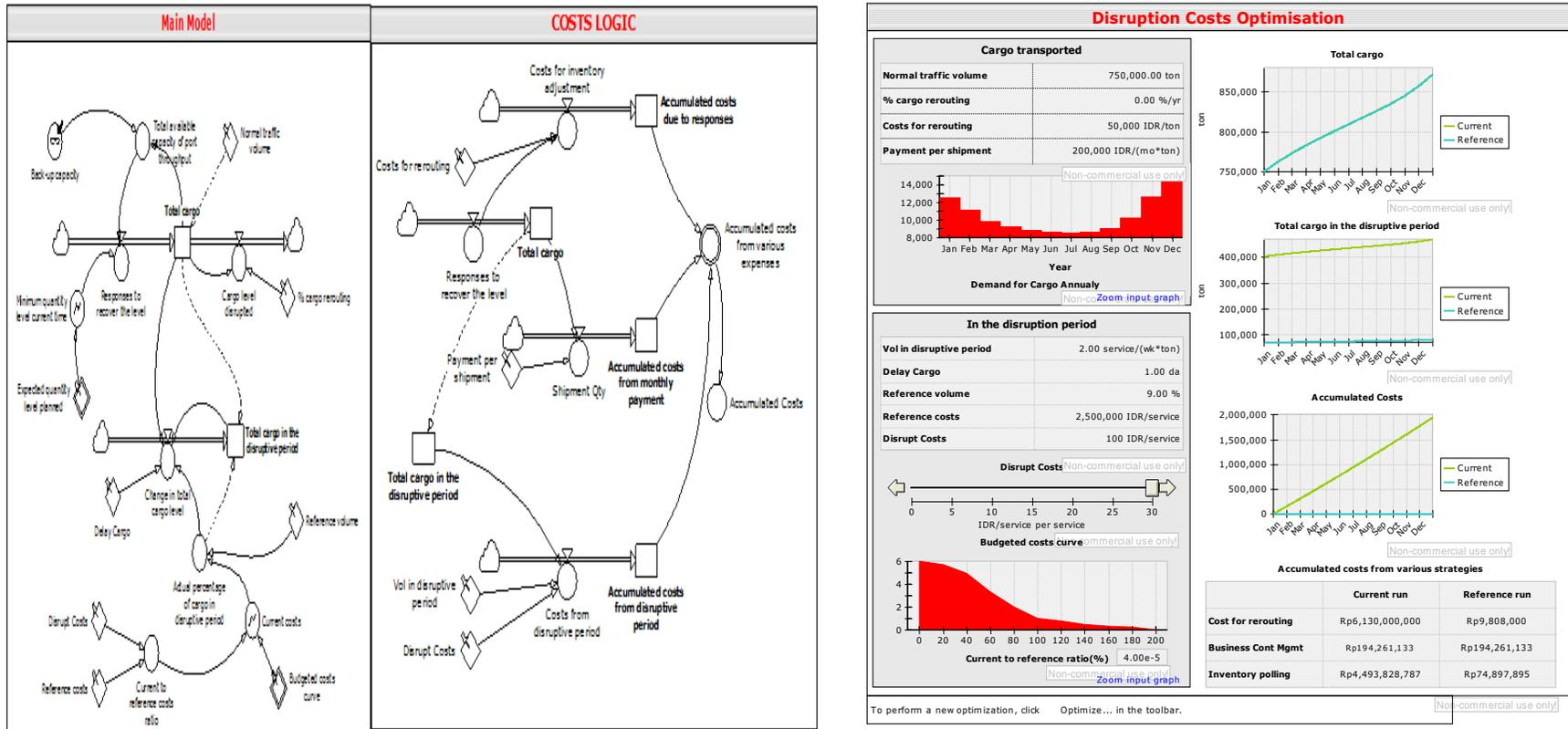
Figure 4. The modeling concept of main model and costs arrangement using Powersim 8.
